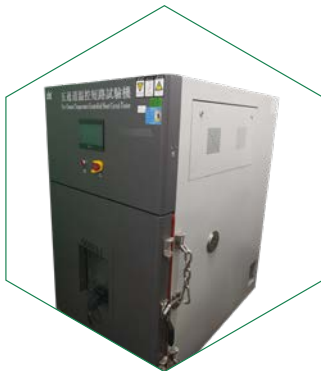
Short Circuit Test
