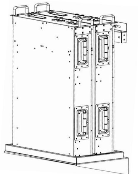
3 Insert the main body into the base components, and fix both sides with 4 screws.
