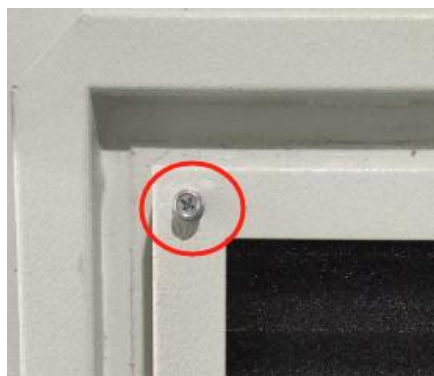
Figure 7.1 Guard Plate Bolt
