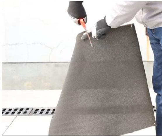
Figure 7.2 Clean Dust-Proof Screen Mesh
