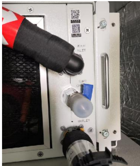
Figure 7.7 Liquid cooling machine injection port
