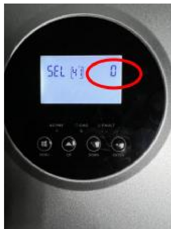
Figure 4. Inverter Program 41 Interface
